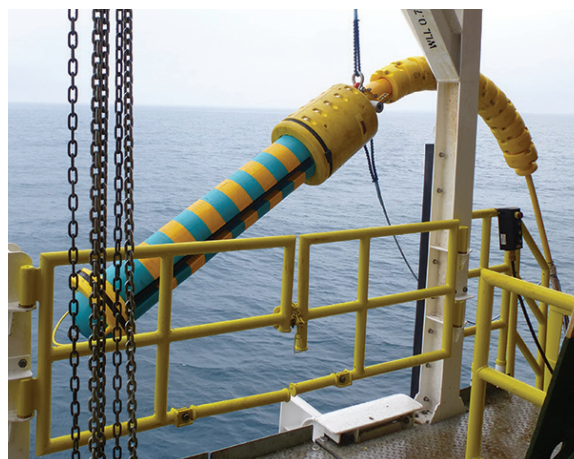
RECOVERY TIME The RetroSAM™ while hoisted onto the recovery porch.
